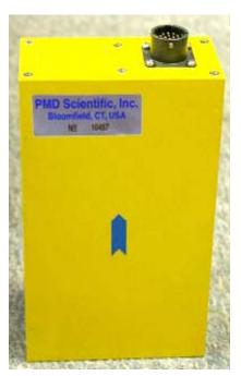
This unique instrument has been developed for the US Department of Energy for use as a wide passband highly sensitive vibration sensor in the beam focusing servo-system of linear super-colliders (very high energy particle accelerators). As such this sensor has been highly radiation hardened and designed to function normally in extremely strong magnetic fields – up to 6 Tesla.
