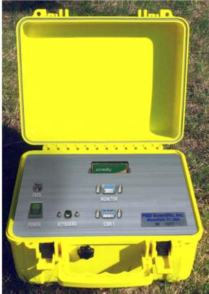
This extremely versatile high-resolution seismic data acquisition system can be configured from 4 to 32 channels, all operating synchronously up to 2,000 samples per second.
